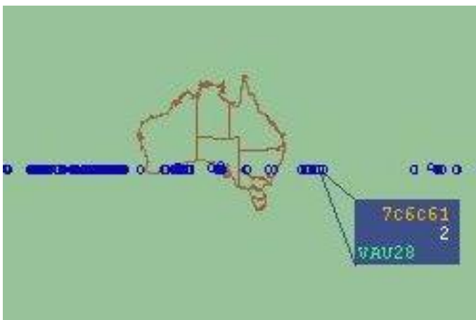
Figure 1 - Track Jumping problem with TPR901
